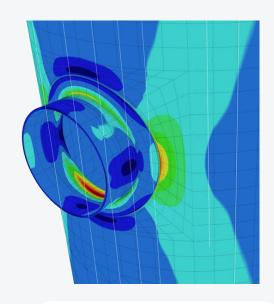
Includes built-in FEA capabilities for nozzles and expansion joints.
